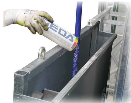
Fig. 5 Adding talcum powder to the cable bin
